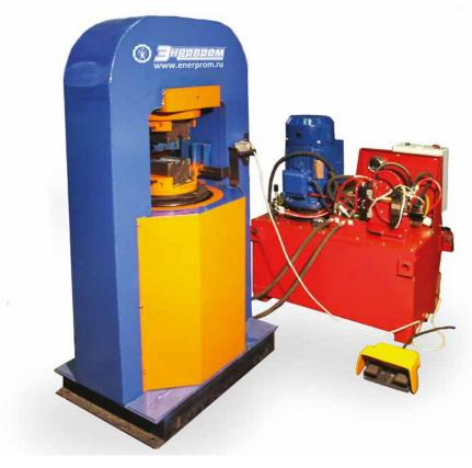
with crimped aluminum alloy plugs and provide the geometry of the pressed plug with guaranteed removal of the flare due to the rigid structure, the required standard force and the exact positioning of the matrices.
